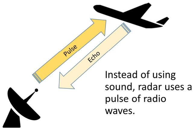
*Q: if  $c_0$  is the speed of light and  $\Delta t$  is the time between the pulse being transmitted and the echo received, write an equation to find the distance to the plane.*
