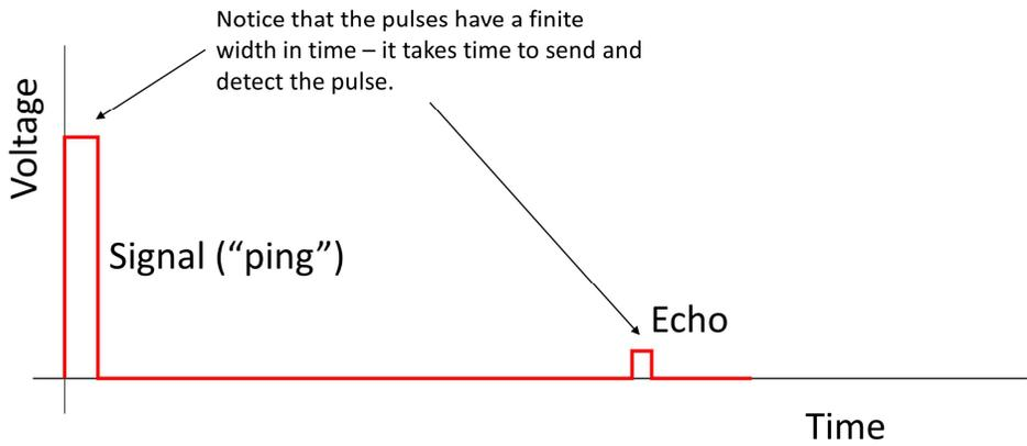
The voltage of the signals will be proportional to the radar energy being transmitted and received. Note that the echo energy is much lower than the ping energy. This means that you should probably consider transmitter power and receiver sensitivity – what's the lowest echo energy the receiver can detect? What is the ratio of transmitter power to receiver sensitivity?
