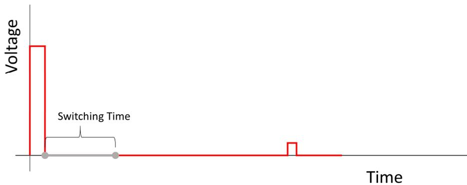
During the switching time the radar station is blind – it cannot detect anything that is within that switching time of the ping.
