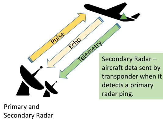
Primary radar sends a ping and waits for the echo. Secondary radar refers to a device on the aircraft called a transponder. The transponder on the airplane listens for the primary radar ping. When it detects the ping it responds with a packet of data that includes the aircraft's identification, altitude, location, bearing, velocity, etc. What we call the radar system has a second receiver that is listening for the telemetry data from the aircraft's transponder.
